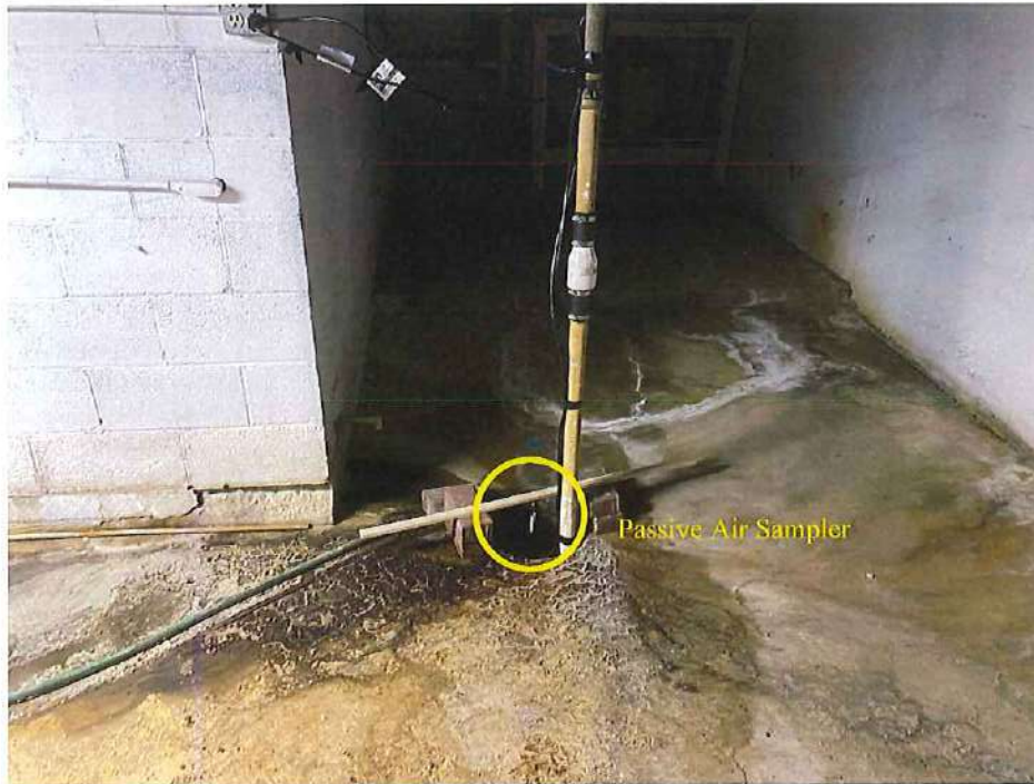
Photo 9: "Sump" passive air sampler deployed at surface of sump. View to north. (July 7, 2022)
