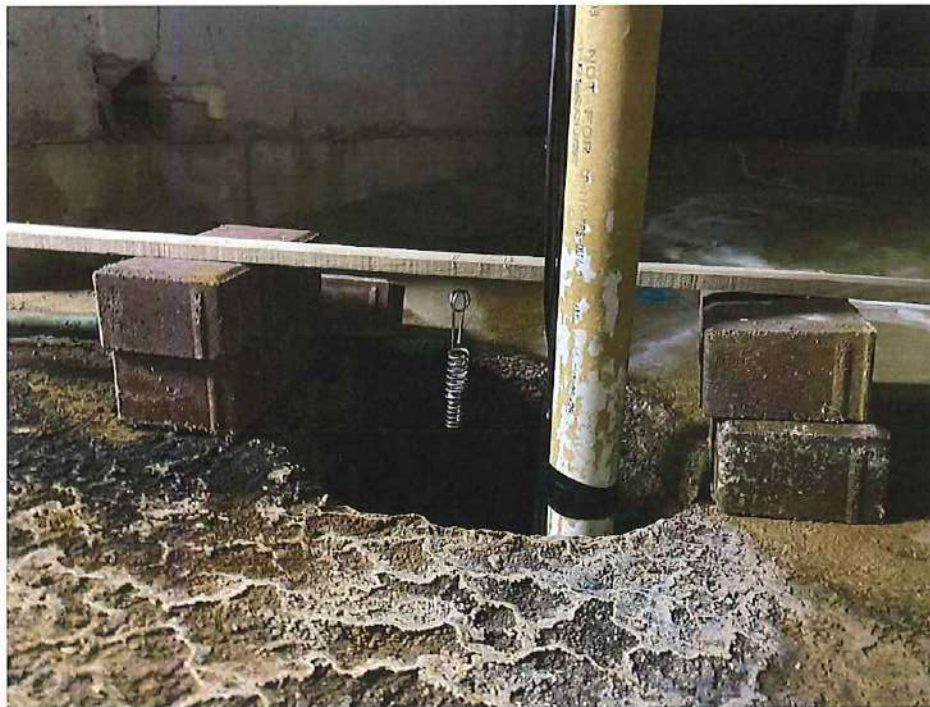
Photo 10: "Sump" passive air sampler deployed at surface of sump. View to northwest. (July 7, 2022)
